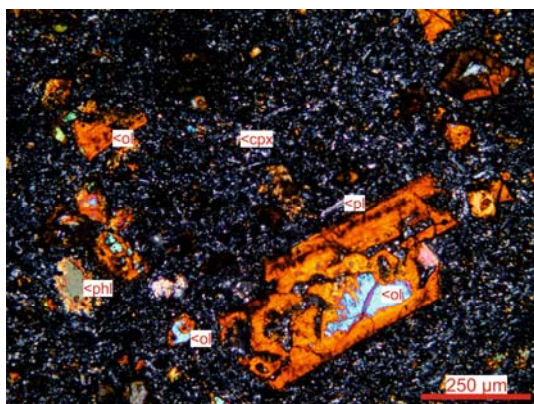
Fig. 4.: Polarizing microscopic photo of NUH-V1 basalt flake with olivine (ol) phenocrysts with fresh core and iddingsitic rim, plagioclase (pl), augitic pyroxene (cpx) and phlogopite (phl) in the completely crystallized groundmass (crossed nicols)
