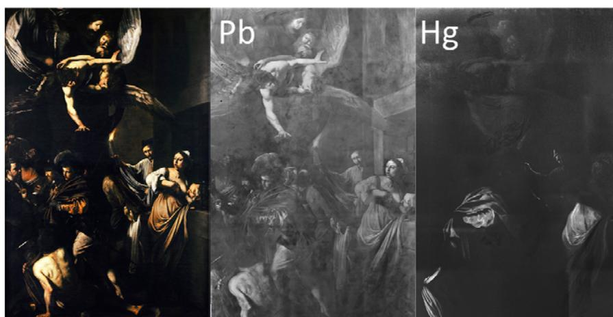
**Fig. 2.:** Pb and Hg elemental maps obtained by applying the MA-XRF technique on "Seven Works of Mercy" by Caravaggio
