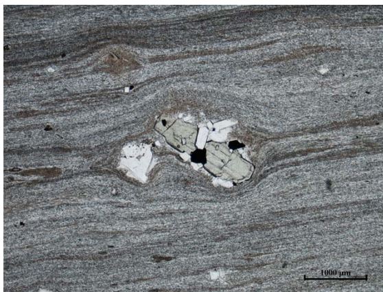
Fig. 7.: Thin section microscopic photos (1N) of C3 type obsidian – aggregate in the fluidal type of matrix
