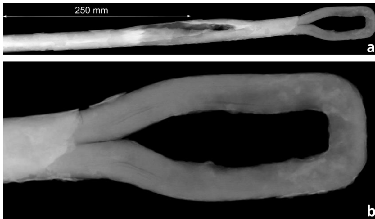
Fig. 11. Neutron imaging study of a wrought iron tie-rod (Milan Cathedral, Italy), (a) The image of the long rod created by as a mosaic of overlapping tiles shows a damaged part and gives some hints about the fabrication technique, (b) the elongated cracks in the material of the long rod are well recognizable.
