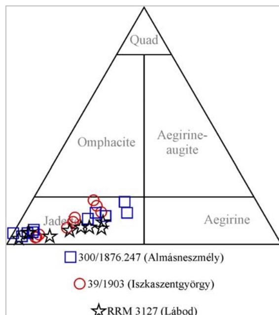
**Fig. 19.:** Pyroxene compositions in iron jadeites. All of results fall to the jadeite field, however compositions are varying between iron poor and iron rich jadeites.
