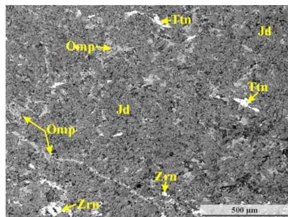
**Fig. 5.:** Typical texture of jadeitites: small amount of omphacite is scattered among jadeite. According to the textural characteristics, omphacite was formed in the latest stage of metamorphism in this sample (300/1876.264, Bakonypéterd).
