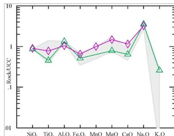
**Fig. 8.:** Bulk-rock compositions of jadeite samples normalized to UCC by McLennan (2001). Results showing very well the correspondence to jadeite compositions by D'Amico et al (2003). Differences in compositions are possibly caused by varieties in omphacite content of the samples.
