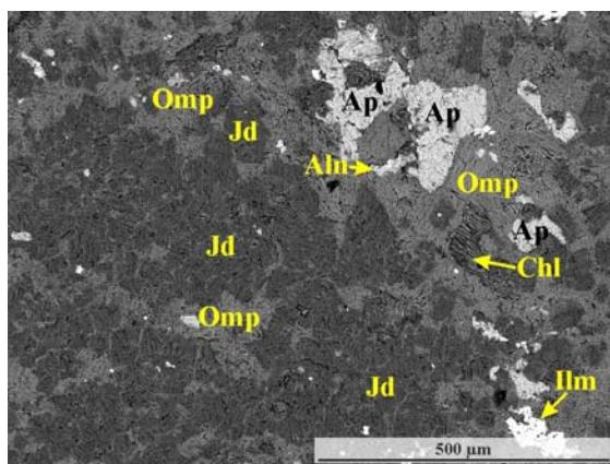
**Fig. 13.:** Textural view of an iron-mixed jade with accessory and retrograde minerals. Sample Olad-329
