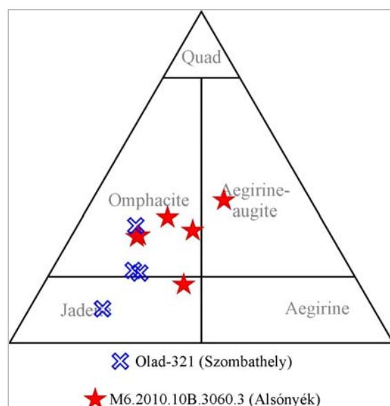
**Fig. 26.:** Pyroxene compositions in the iron eclogite samples. Most of the compositions fall into the omphacite field, however there are some jadeite and aegirine-augite összetételű mérések.
