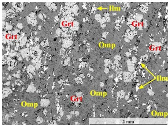
**Fig. 24.:** Typical texture of iron eclogites with accessory minerals and large amount of garnets. Moderate inhomogeneity of pyroxenes can be observed on this sample (M6.2010.10B.3060.3, Alsónyék). Foliation is visible on the placements of ilmenite crystals.
