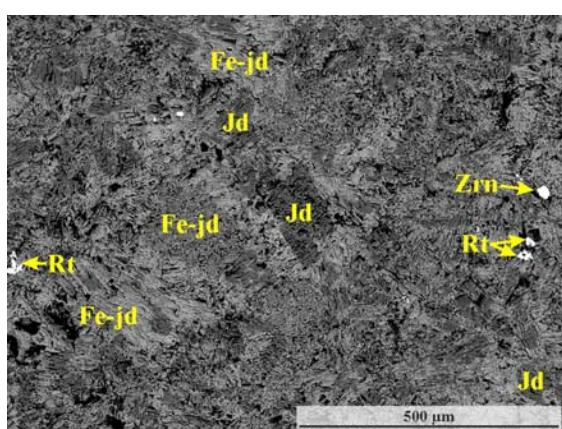
**Fig. 18.:** Zoned pyroxenes with jadeite core and iron-jadeite rim. Sample 3127 from Lábold.
