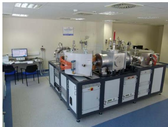
**Fig. 3.:** The MICADAS AMS system installed at Debrecen (courtesy Dr. M. Molnár).
