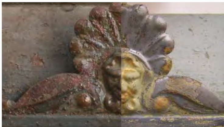
Fig. 19. The antefix of the aquarium a) before conservation and b) after blasting with abrasive glass beads
