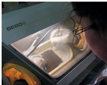
Fig. 8. Cleaning the iron parts of the mail by blasting them with tiny glass beads
